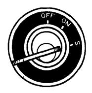
Should the engine not start even when the starter switch is left at "S" position for 10 seconds, take your hand off the starter switch for 30 seconds, and then attempt to start the engine again by sufficiently preheating the glow plug. The starter motor should never be allowed to run for more than 30 seconds at a time.
