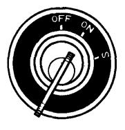
During engine operation, do not turn the key to "S" position. This may damage the starter motor.
