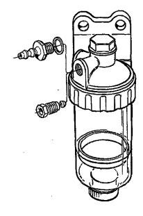
If a water trap type filter (see page 13) is not interposed between the fuel tank and engine lift pump, any entrained water will tend to lay in the bottom of the electric lift pump. Internal metal parts of the lift pump will rust. Particles will pass on to filters and eventually to injection pump and injectors with damaging and expensive results. It is well to remember that water damage to the fuel system is not covered by warranty!
